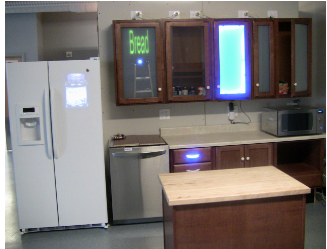
Figure 1 The experimental settings used in this study. This is the kitchen test-bed implemented with sensors and prompts. The image on the refrigerator showing that the jelly is in the refrigerator is an example of the image prompts. The glass of the second left cabinet becoming transparent is a smart glass prompt. The lighted door of the middle cabinet and the glowing handle of the top drawer show examples of the light prompts.
